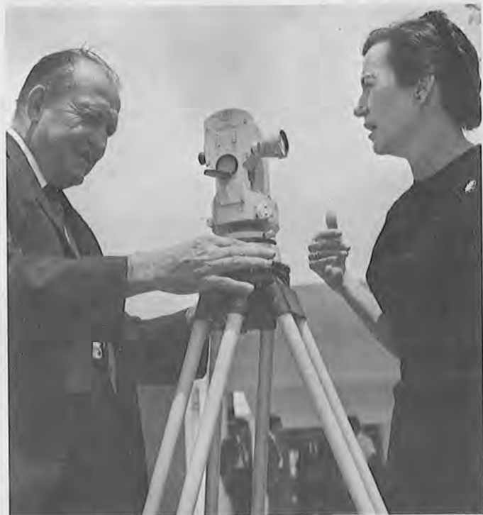
Staying informed on the latest developments in surveying technology is part of Mrs. Edwina Polk's role as practicing engineer and educator. Here she examines a new Zeiss Theodolite being demonstrated by Keuffel & Esser representative Dan B. Glisson. Theodolites are the instruments likely to become the most widely used in American surveying, Mrs. Polk believes.
