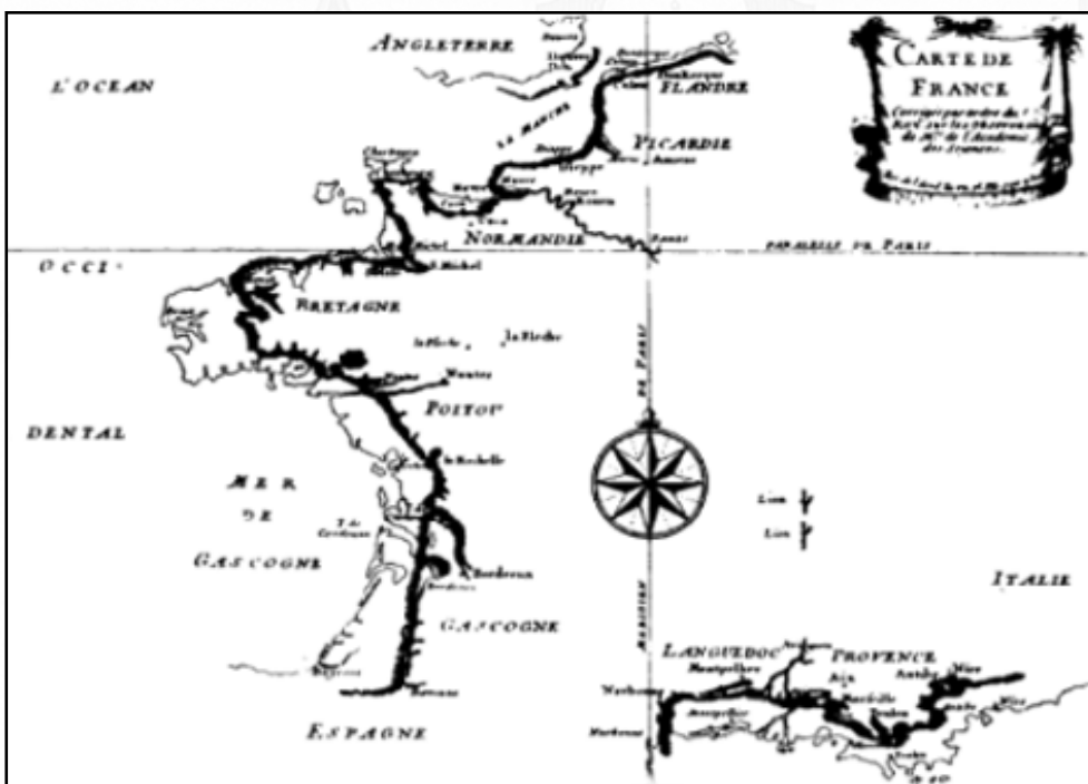
The resurvey of France under Cassini and Picard resulted in the above improved profile ( shaded ). (From The Story of Maps by Lloyd A. Brown.)
