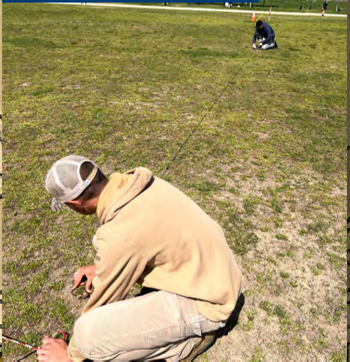
UF Geomatics Students Gabe Hancock and Kenneth Dell working with a 33' Gunter's Chain and Chaining Pins to measure the sides of the parcel in the Geometric Traverse problem.
