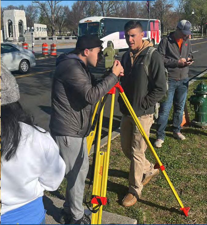
UF Students Gabe Hancock and Kenneth Dell work with a T2 Manual Theodolite to sight the Washington National monument.
