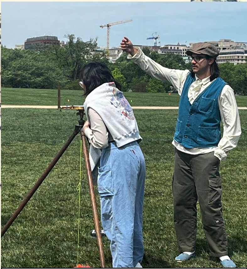
Day 2: UF Student Jacob Suarez aligning the chaining crew while Vanessa Zhao is reading the azimuth on the Compass during the Traverse Exercise. Students were tasked with recording azimuth readings from a 1800s Compass while using a 33' Gunter's Chain to measure the distance between corners.
