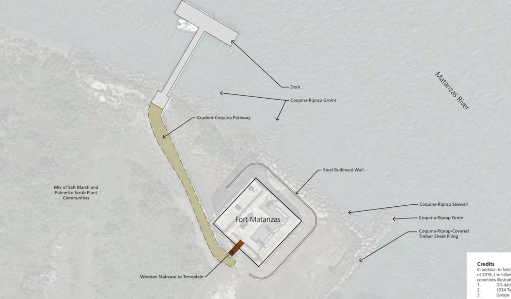
Site plan from the Cultural Landscape Report showing existing conditions at Fort Matanzas, 2019. National Park Service
